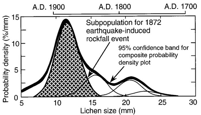
Figure 2. Probability density of lichen size measurements at Knapp's Rock rockfall site in Kings Canyon portrayed as composite plot with 95% confidence band. Amplitude (seismic-shaking index) of 12 mm peak reflects magnitude 7.6 earthquake of 1872 (Lubetkin and Clark, 1988); epicenter was only 50 km from Knapp's Rock.
