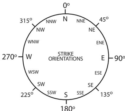
Fault plane solutions also indicate what the **strike orientation** of the fault plane is. In other words, the orientation of the intersection line between the fault and a horizontal surface, such as a flat part of the Earth's surface. This is the orientation you would see if you were flying overhead in an aircraft.
