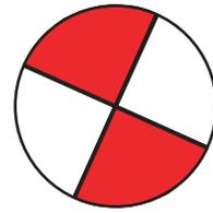
Focal mechanism solutions utilize stereonet representations of fault plane orientations. This is a curved line inside a circle that represents the line of intersection of a plane and the inside of a lower hemisphere, like the inside of a bowl.
