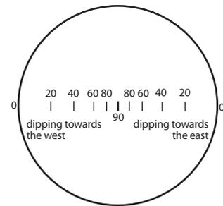
The direction towards which the fault plane is dipping is given by the direction towards which the convex side of the curve is pointing. So for both cases on the right, the fault plane is dipping towards the northeast. Dip directions are always given as compass directions. On the right, the left example shows a fault dip of about  $80^\circ$  NE. The right example shows a fault dip of about  $20^\circ$  NE. Vertical faults and horizontal faults do not have a **dip direction**.
