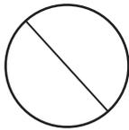
A steeply dipping plane will produce a slightly curved line that passes close to the center of the circle.
