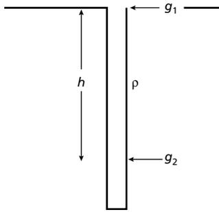
**Fig. 6.14** Density determination by subsurface gravity measurements. The measured gravity difference  $g_1 - g_2$  over a height difference  $h$  can be used to determine the mean density  $\rho$  of the rock separating the measurements.
