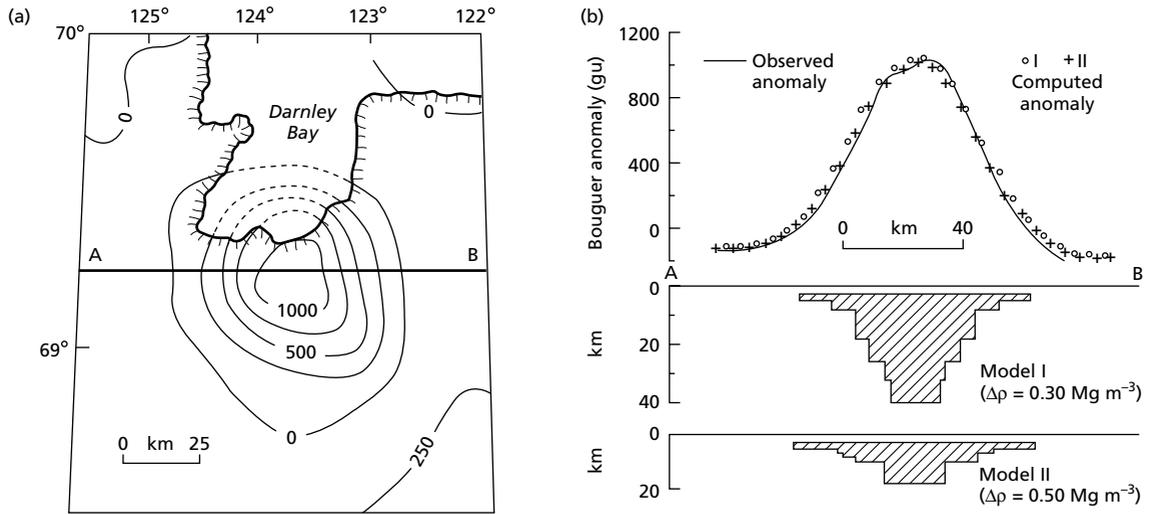
**Fig. 6.20** (a) The circular gravity anomaly at Darnley Bay, NWT, Canada. Contour interval 250 gu. (b) Two possible interpretations of the anomaly in terms of a model constructed from a suite of coaxial vertical cylinders. (After Stacey 1971.)
