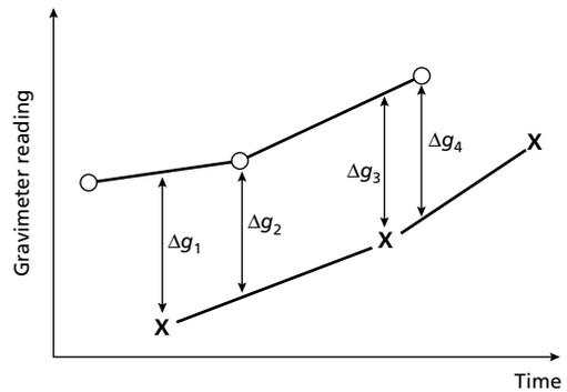
**Fig. 6.9** The principle of looping. Crosses and circles represent alternate gravimeter readings taken at two base stations. The vertical separations between the drift curves for the two stations ( $\Delta g_{1-4}$ ) provide an estimate of the gravity difference between them.
