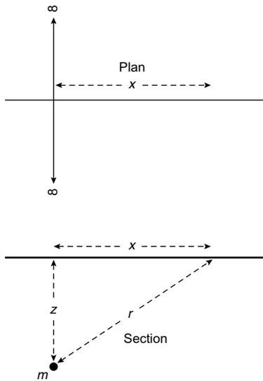
Fig. 6.7 Coordinates describing an infinite horizontal line mass.
