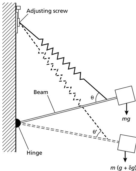
Fig. 6.2 Principle of the LaCoste and Romberg gravimeter.
