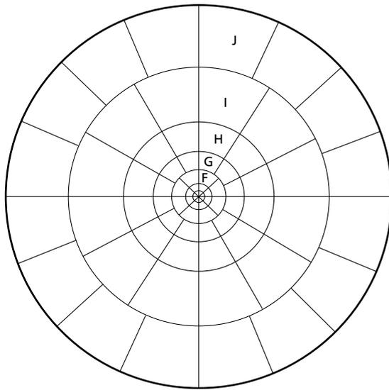
**Fig. 6.13** A typical graticule used in the calculation of terrain corrections. A series of such graticules with zones varying in radius from 2 m to 21.9 km is used with topographic maps of varying scale.
