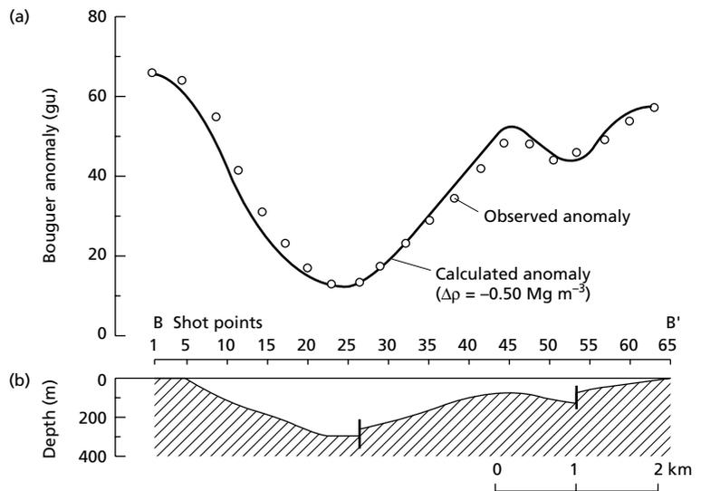
**Fig. 6.29** Profile B-B', Taltal area, Chile (see Fig. 6.28 for location). (a) Observed Bouguer anomaly and calculated anomaly for a model with a density contrast ( $\Delta\rho$ ) of  $-0.50 \text{ Mg m}^{-3}$ . (b) Gravity interpretation. (After Van Overmeeren 1975.)
