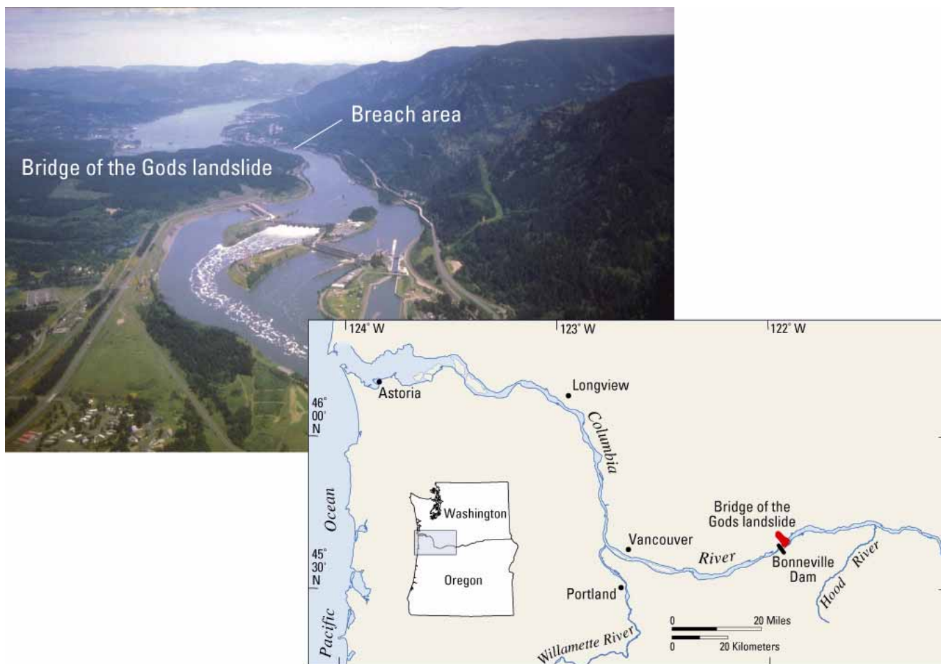
Figure 4. The Bridge of the Gods landslide slid down from the north wall of the Columbia River Gorge sometime between 1400 and 1465 A.D., blocking the Columbia River to a depth of 70–80 meters. Breaching of almost the entire thickness of the landslide dam caused a flood of about 220,000 cubic meters per second, about six times larger than the largest meteorological flood of the last 150 years. Deposits from the flood form a distinctive marker bed all the way to the Pacific Ocean. The last remnant of the dam was bouldery Cascade Rapids, the namesake of the Cascade Range, now drowned in the pool behind the 24-meter-high Bonneville Dam. (Photograph courtesy of the U.S. Army Corps of Engineers)
