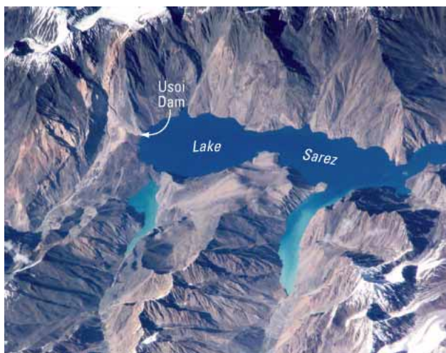
Usoi Dam in Tajikistan, formed by a landslide in 1911, created 16 cubic-kilometer Lake Sarez, the largest lake in the world resulting from a landslide. Five million people live in the valleys downstream of the dam. Even partial breaching of the dam could cause catastrophic flooding. Complete failure of the dam could result in the deadliest natural disaster in human history. (Photograph courtesy of NASA)
