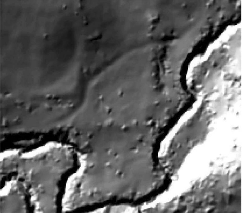
**Fig. 5.** Portion of a bare earth shaded relief image showing artefacts (bumpy texture) in deciduous forest areas. These artefacts are LiDAR elevations classified as bare earth, but probably are from tree trunks, branches or understorey close to the ground and classified as bare earth by the vendor's algorithm.
