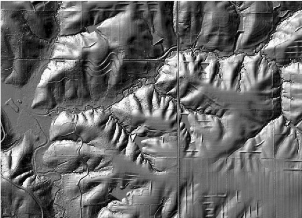
**Fig. 4.** Portion of the bare earth shaded relief image of the Lake Darling watershed showing natural and man-made features readily apparent in the LiDAR data. Natural and man-made drainage features, roadbeds, fence lines and tillage patterns are readily visible.
