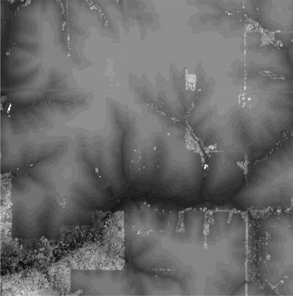
**Fig. 1.** Grey scale image consisting of 3.3 million LiDAR first return LiDAR points. First returns indicate the tops of trees and buildings, as well as bare ground in open areas. White areas are data voids where no returns were recorded, usually from non-reflecting water surfaces.
