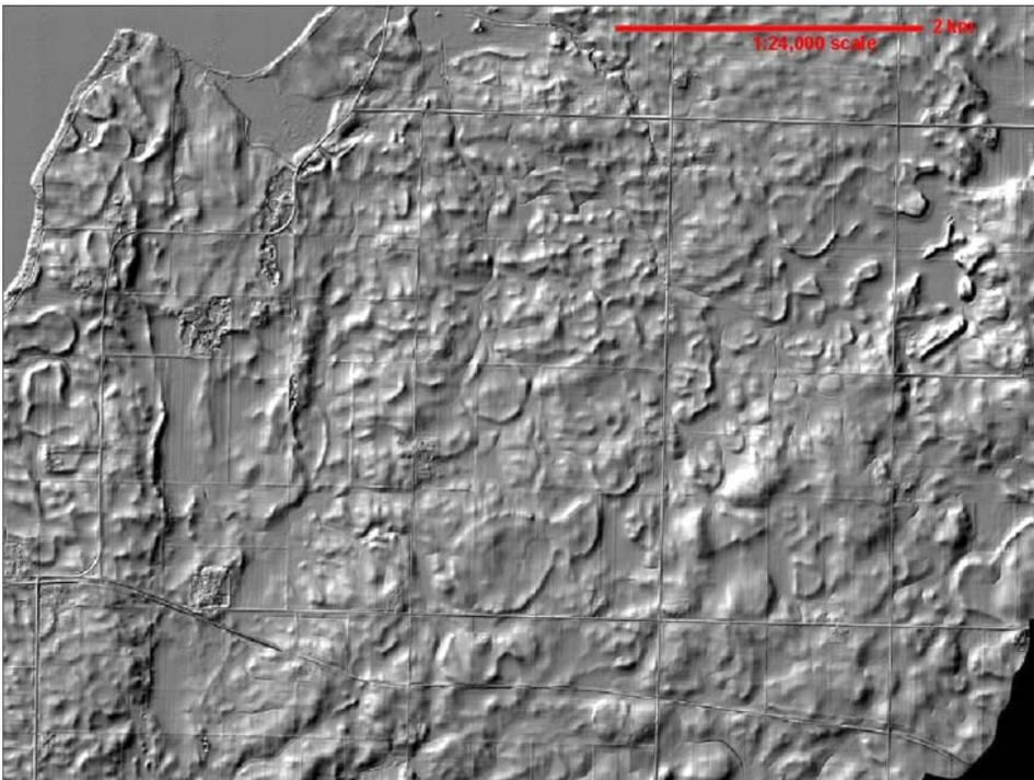
**Fig. 14.** Portion of a LiDAR-derived shaded relief image of the same area of glacial terrain near Spirit Lake in Dickinson County, Iowa. Notice how the shapes of subtle, low relief glacial features are now readily apparent.
