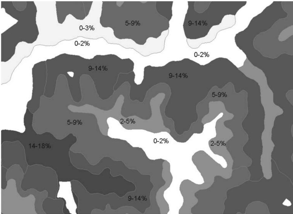
**Fig. 6.** Soil survey soil polygons shaded by slope class range: light shades are lower slopes and darker shades indicate steeper slopes.
