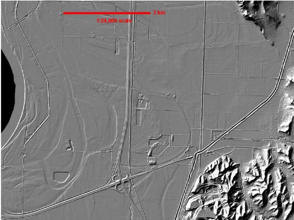
**Fig. 16.** Portion of a LiDAR-derived shaded relief image of the same area on the Missouri River Floodplain. Notice the much finer detail showing the interstate cloverleaf, river meander scars, borrow pits, and a ditch and levee system. Editing by the vendor removed the bridge deck. LiDAR DEM obtained from the Pottawattamie County GIS Department.
