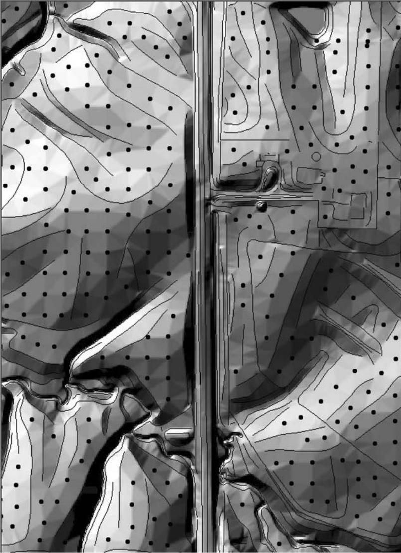
**Fig. 9.** A  $0.4 \times 0.6$  km portion of shaded relief of a digital terrain model derived from low-altitude aerial photographs. The black dots are elevation mass points and the black lines are break lines.
