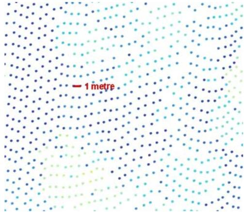
**Fig. 2.** An area in the middle of a LiDAR flight line. LiDAR point spacing is around 1 m at the centre of back-and-forth scans.
