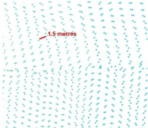
**Fig. 3.** An area of two adjacent LiDAR flight lines. The point spacing is highly variable at the edges of flight lines. Some points are less than 1 m apart at the end of one and beginning of the next scan, while the distance between points in different sets of scans can be as much as 1.5 m apart.
