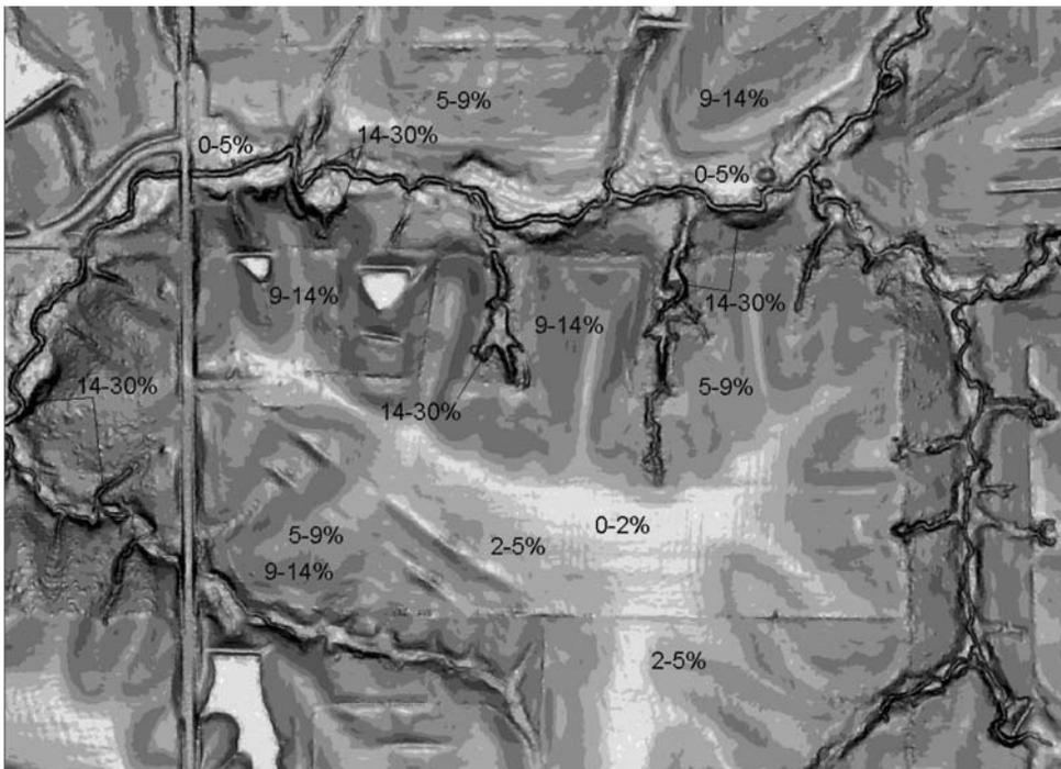
**Fig. 7.** Slope class ranges derived from Lake Darling LiDAR data. While low slope areas on LiDAR look similar to the soil polygons, LiDAR more clearly represents steep slopes such as gullies and stream channels.
