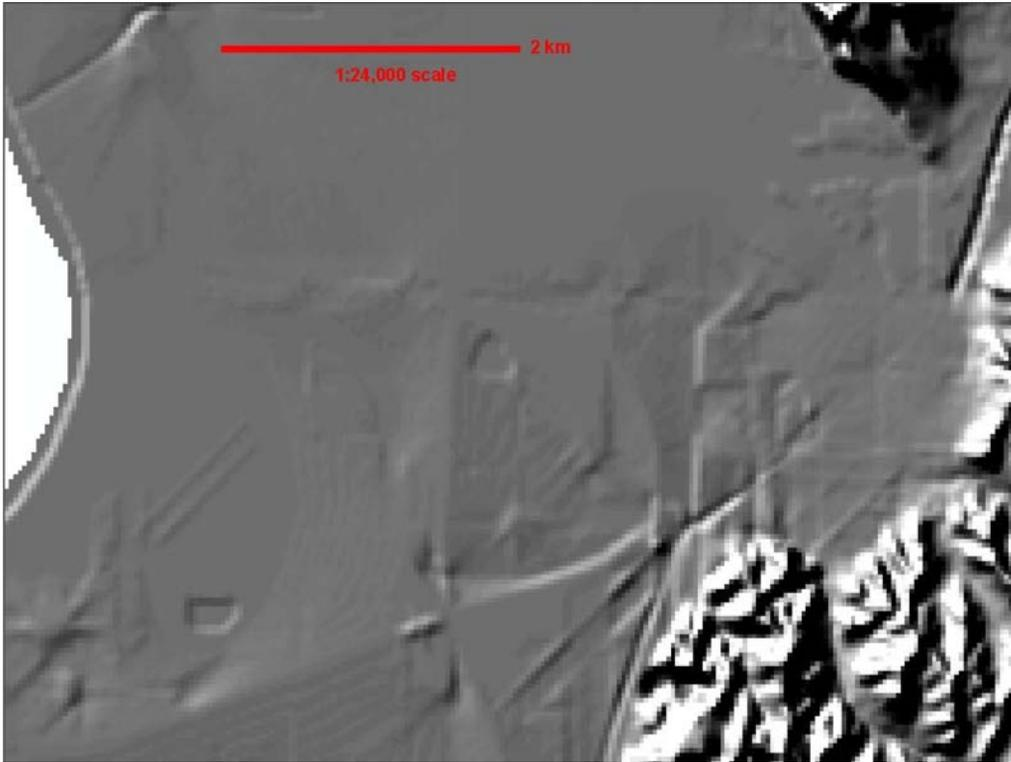
**Fig. 15.** Portion of a shaded relief image showing the Missouri River floodplain north of Council Bluffs, Iowa. The shaded relief image was created from a 30 m resolution DEM from the NED. Notice the cross-shaped features that are artefacts of the interpolation of the original 10 ft contours from USGS topographical maps.
