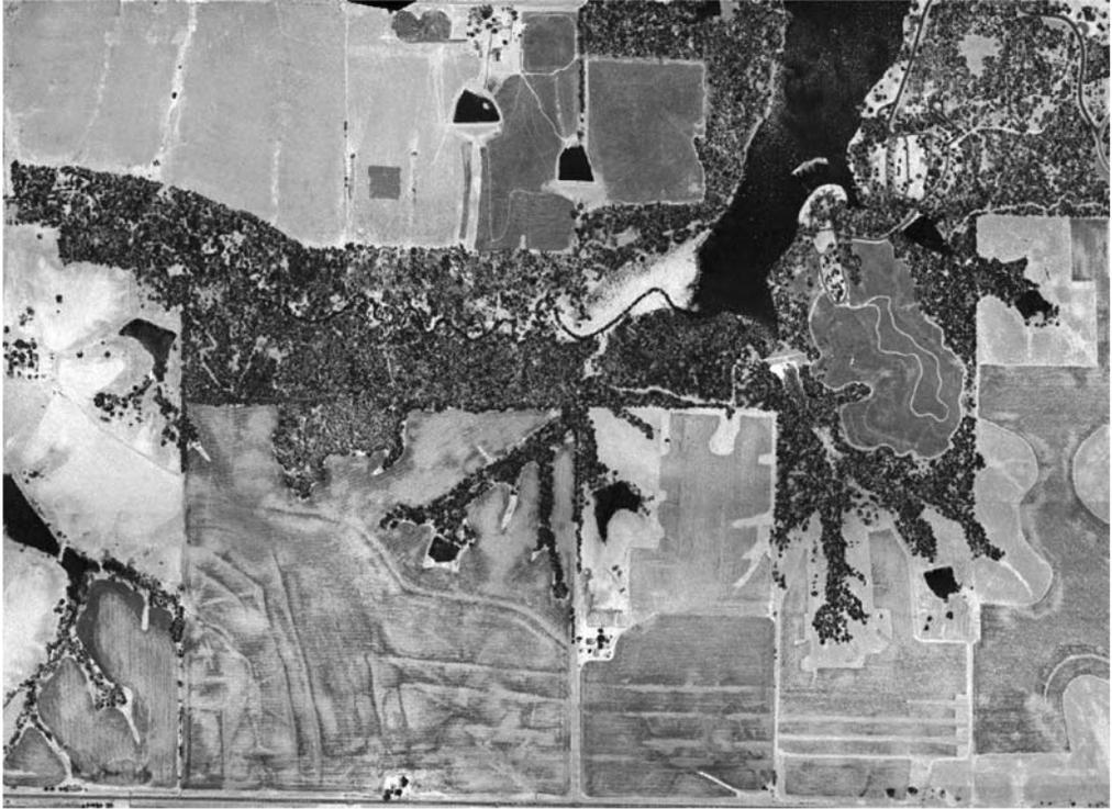
**Fig. 8.** Portion of a LiDAR intensity image of the Lake Darling watershed, constructed from bare earth return intensity values.
